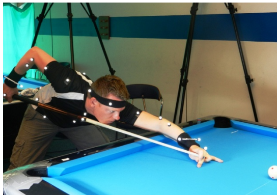
Pic. 1. Reflective markers attached to skin to identify bony landmarks and the 3D motion of body segments.
